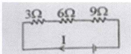
Calculate the electric resistance of this electric circuit.
